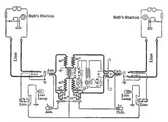
FIG. 179. Diagram of a pair of Circuits in a Common Battery Telephone Exchange.
